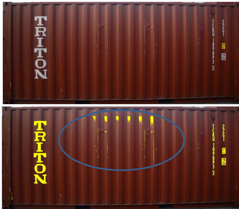
Fig. 14 Original container image with damages (top). Damages marked with circle (bottom)
