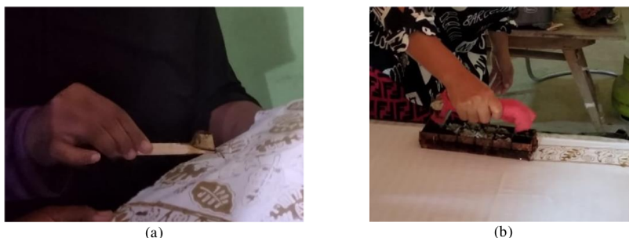
Figure 1. The process of making batik using tulis (a) and cap (b) method
