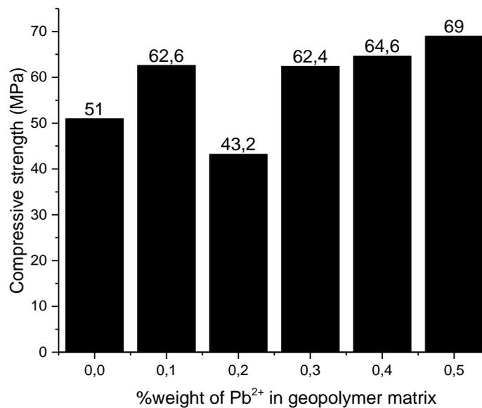
Figure 4: The compressive strength of geopolymer with various weight percentage of Pb<sup>2+</sup>
