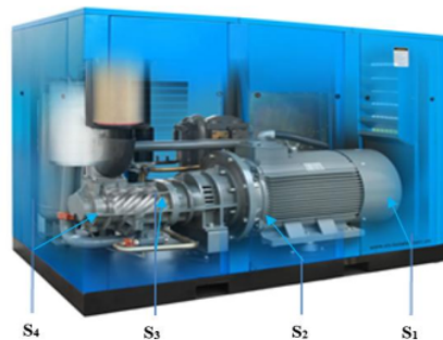
Figure 2. Simplified representation of sound source from the compressor machinery used in this study
